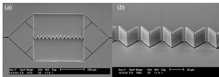
Figure 2. SEM pictures of the microfabricated funnel wall. (a) Top view. (b) Side view of the 20  $\mu\text{m}$  etch depth.
